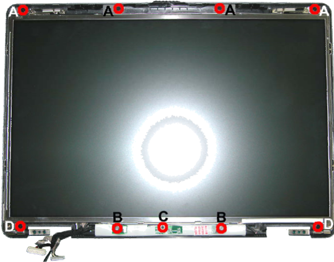
Fig. 27 Removing the LCD panel screws
